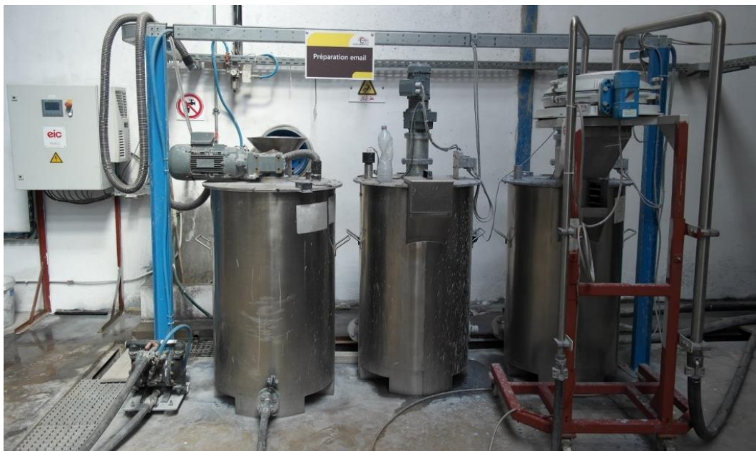
Figure 64 enamel coating preparation mixing unit [3]
