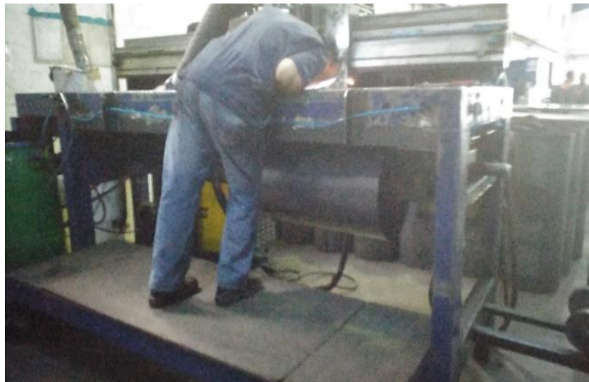
Figure 46 Linear welding of inner tank [3]
