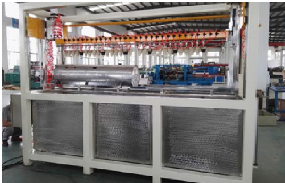
Figure 60 Water bath for leakage test using compressed air
