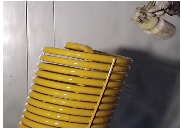
Figure 87 Heat exchanger tubes outer coating [10]
