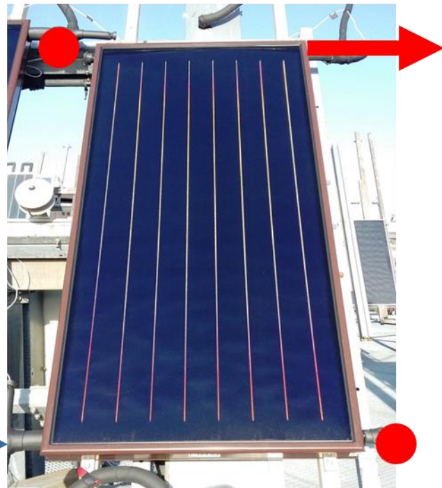
Figure 130 Water flow direction for exposure test (internal shock) [11]
