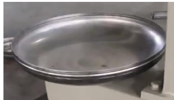
Figure 50 Rounding of inner tank end covers by used of piston
