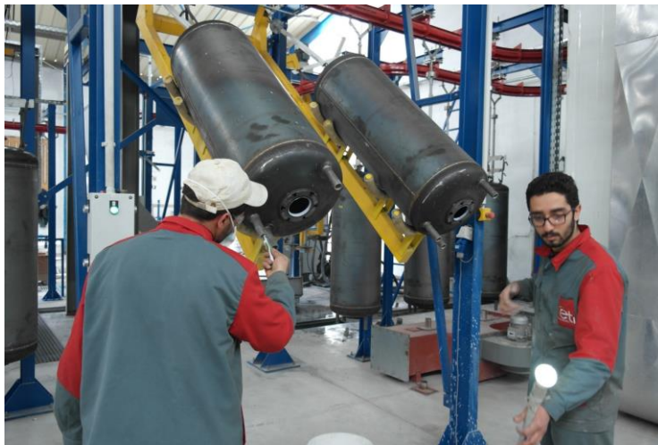
Figure 74 Visual inspection of internal enamel coating [3]
