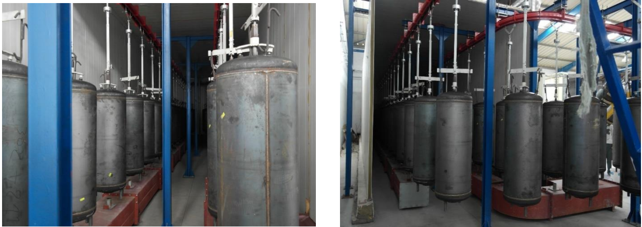
Figure 66 Tanks drying tunnel process [3]
