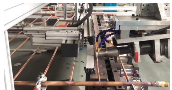
Figure 102 Example setup of the roughen treatment process [4]
