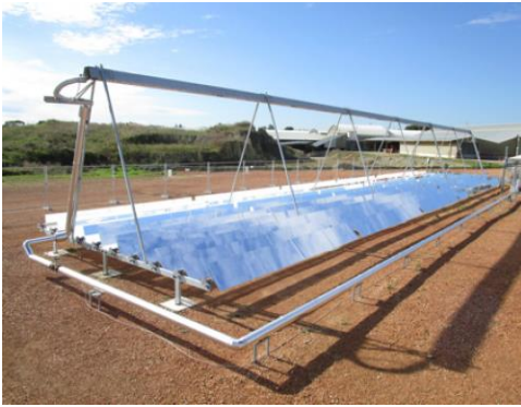
Figure 16 Fresnel collector, Soltigua
