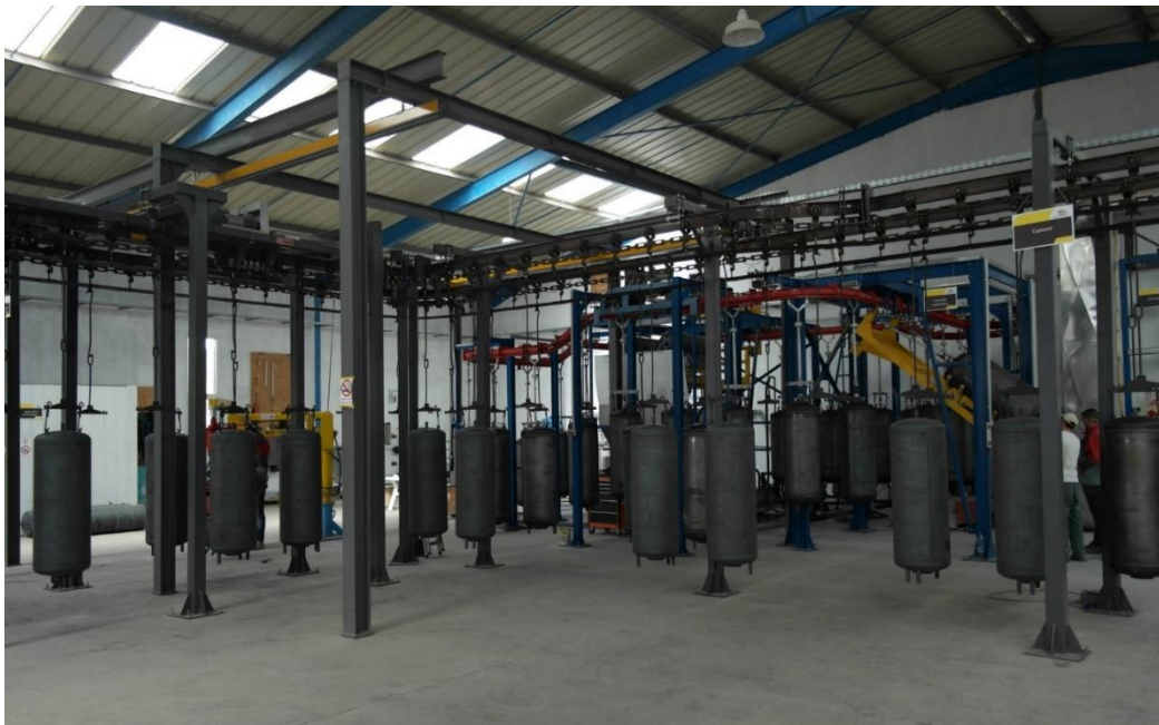
Figure 71 Enamel coated tanks cooling process [3]
