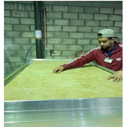
Figure 107 Insulation placement inside the frame casing [3]
