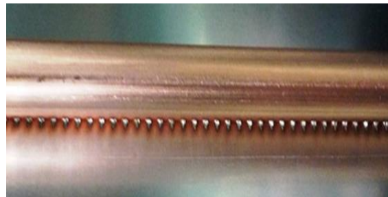
Figure 105 Laser welding of riser tubes and absorber sheet [4]
