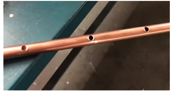
Figure 97 Punched holes along header tube length [4]
