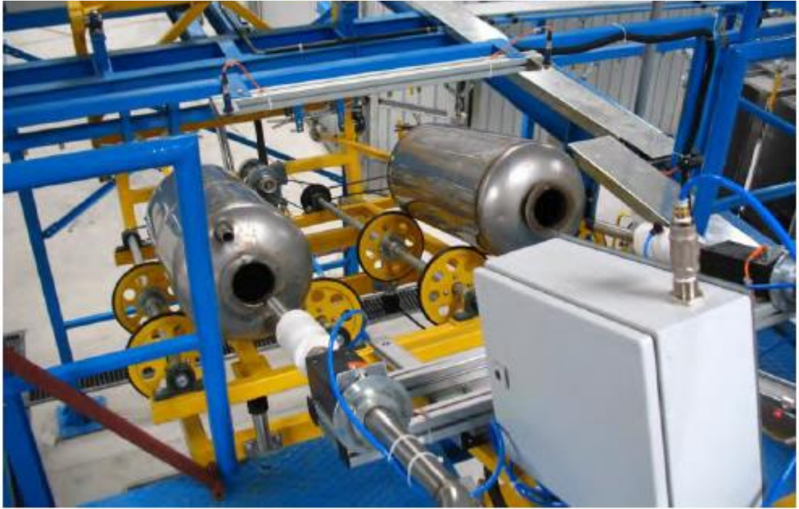
Figure 67 Enamel coating injection process (Flooding ) [7]
