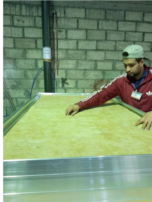
Figure 109 Scratch system in assembly of flat plate collector [3]
