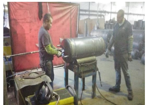
Figure 57 Quality control of circular welding [3]
