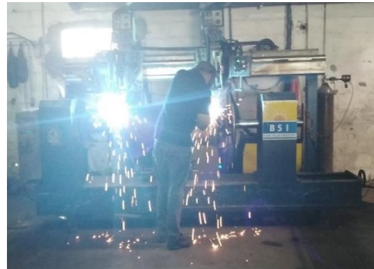
Figure 55 Circular welding using Automatic MIG welding machine [3]
