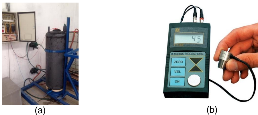
Figure 73 Enamel coating thickness testing (a) dielectric intensity and (b) ultrasonic thickness detector
