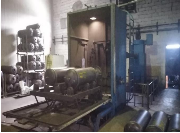
Figure 62 Inner tank sand blasting process (preparation and loading) [3]
