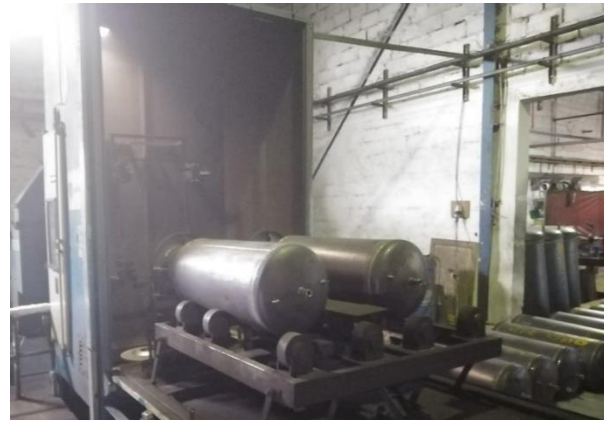
Figure 62 Inner tank sand blasting process (preparation and loading) [3]
