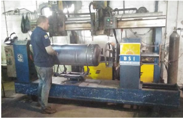
Figure 55 Circular welding using Automatic MIG welding machine [3]
