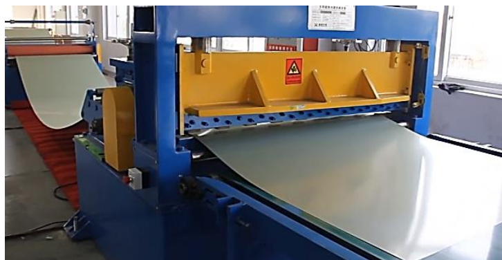
Figure 42 Inner tank sheet cutting [3]
