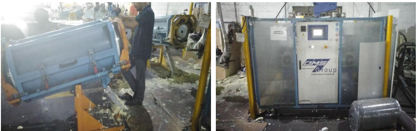
Figure 78 Foam insulation injection machine [3]
