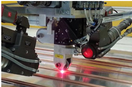
Figure 105 Laser welding of riser tubes and absorber sheet [4]
