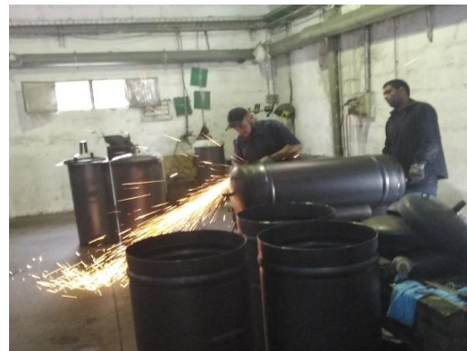
Figure 54 Tack welding and surface cleaning of the circular surface [3]
