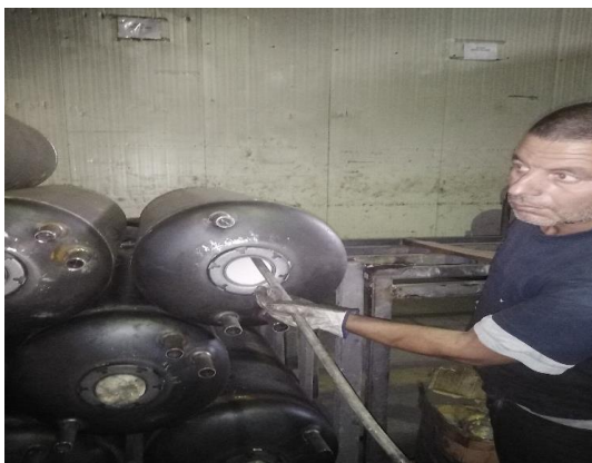
Figure 63 Visual inspection after blasting process [3]
