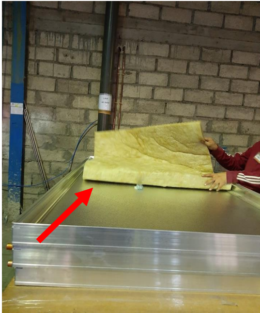
Figure 109 Scratch system in assembly of flat plate collector [3]
