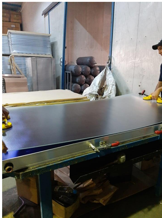
Figure 111 Final assembly of flat plate collector with glass cover [3]
