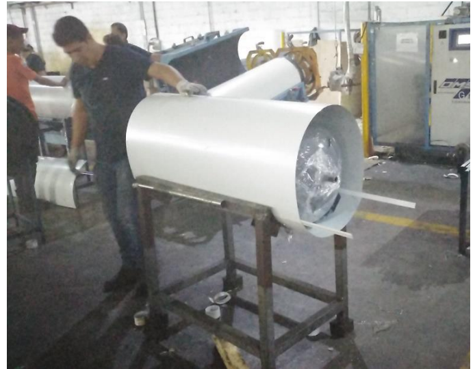
Figure 76 Fixing process of outer tank including (a) packaging with stretch inner tank and (b) fixing separators between inner and outer tanks [3]
