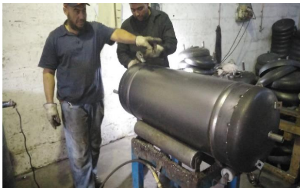
Figure 54 Tack welding and surface cleaning of the circular surface [3]
