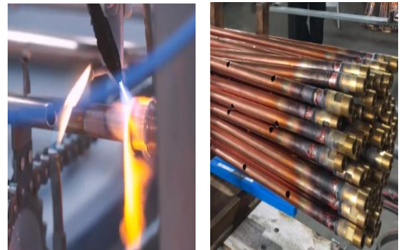
Figure 98 Header tube fitted with connection joints [4]
