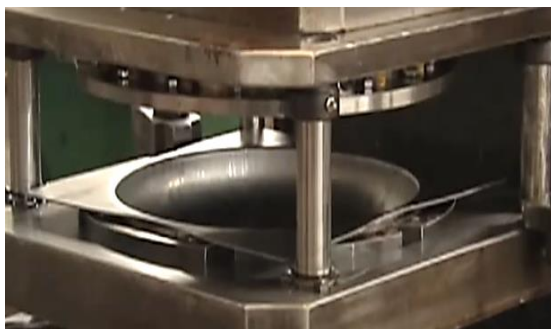
Figure 50 Rounding of inner tank end covers by used of piston
