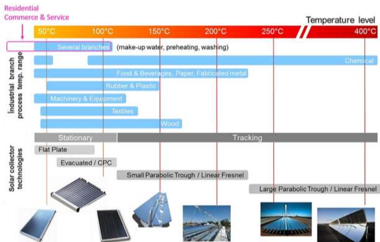
Figure 1.1 Overview of collector types based on their operating temperature and application in industrial, residential and commercial sectors (purple lines) [2]
