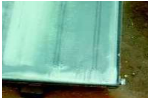
Figure 37: Under glass collector leaking
