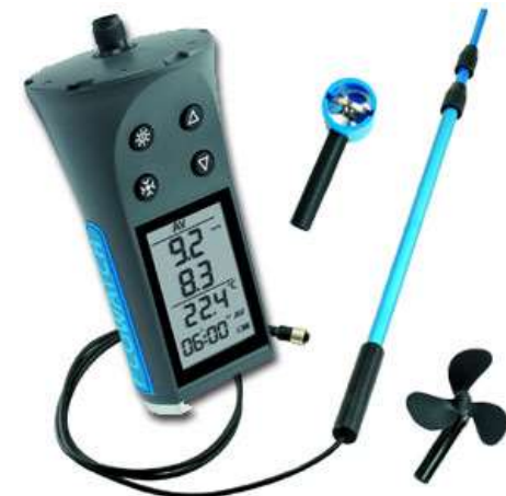
Flowmeter ( for water flow measurement)
